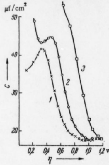
Fig. 2. Differential capacity curves, for the same solutions as in Fig. 1, at a frequency of 5000 cps.
