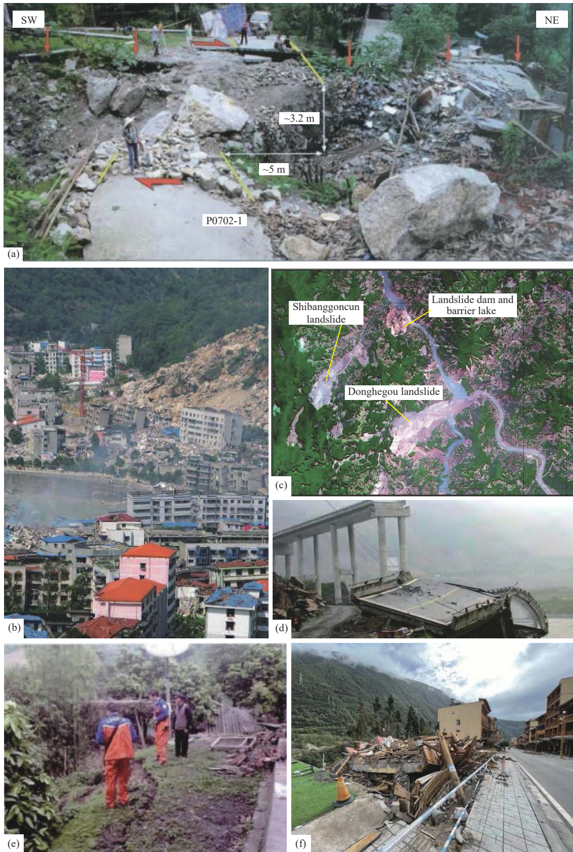
Fig. 2. a–Fracture outcropped in the Shenxigou village, about 3.2 m uplifted road with the about 5 m dextral offset, which generated in the 2008 Wenchuan M_S 8.0 earthquake (Li HB et al., 2008); b– photo of Beichuan county showing the damage caused by the 2008 Wechuan M_S 8.0 earthquake (Tang C and Westen CJV, 2018) ; c–a lots of landslide and barrier lake at Qingchuan county induced by the 2008 Wenchuan M_S 8.0 earthquake (Tang C and Westen CJV, 2018); d–a bridge was destroyed by the 2008 Wenchuan M_S 8.0 earthquake near Yingxiu Town (Tang C and Westen CJV, 2018); e–an arc tissue at Lingguan town generated in the 2013 Lushan M_S 7.0 earthquake around the rural building (Hong HC et al., 2013); f–crushing damage of buildings at Moxi town were destroyed by the 2022 Luding M_S 6.9 earthquake.
