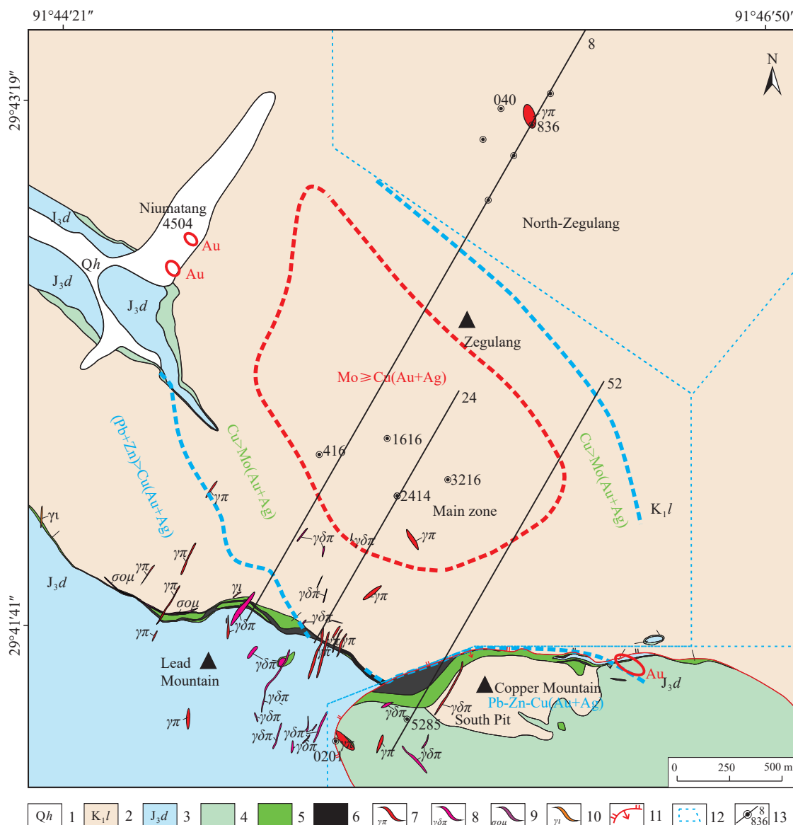
Fig. 2. Geology of the Jiama deposit showing the distribution of metal mineralization (modified from Lin B et al., 2019). 1–Quaternary sediment; 2–Sandstone, slate, and hornfels of the Lower Cretaceous Linbuzong Formation; 3–Limestone and marble of the Upper Jurassic Duodigou Formation; 4–Skarnized marble; 5–Skarn; 6–Skarn orebody; 7–Granite porphyry dike; 8–Granodiorite porphyry dike; 9–Quartz–diorite porphyry dike; 10–Aplite dike; 11–Slip fault; 12–Range of different ore zone; 13–Borehole and section
