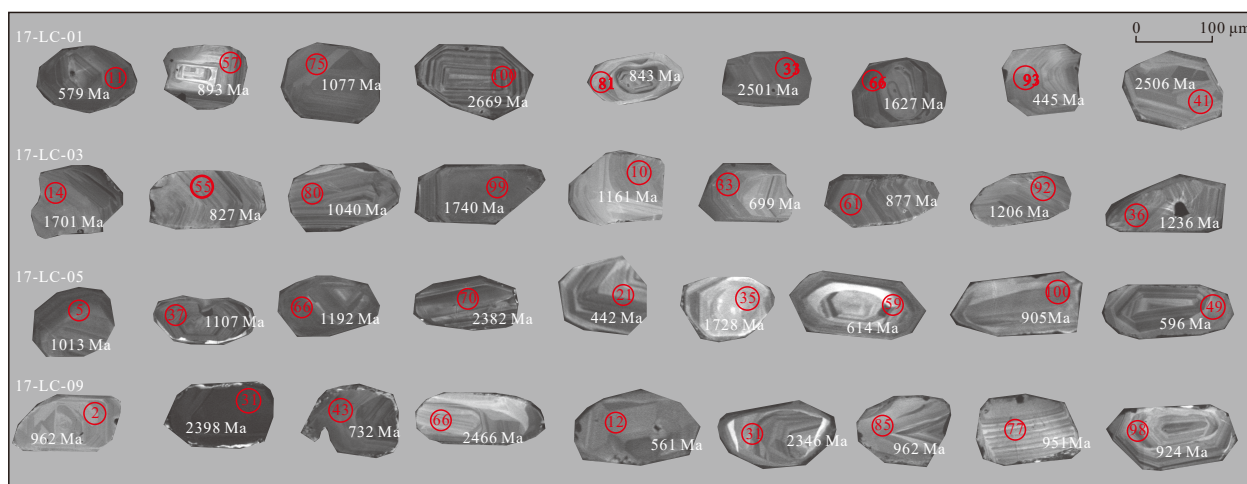
Fig. 5. Cathodoluminescence images of representative zircon grains showing analytical spots of U–Pb age.
