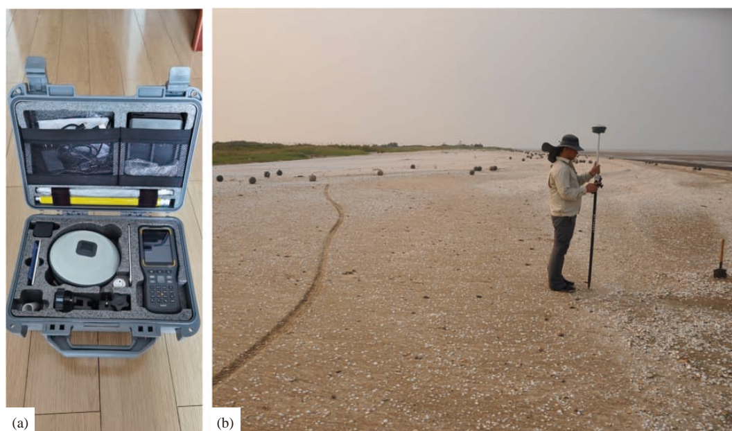
Fig. 5. Field measurement for elevation of the tidal flat; a–measuring instrument (iRTK5); b–field measurement.
