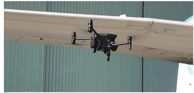
Fig. 9. A DJI M30 drone is used to inspect a real aircraft surface based on the generated viewpoints.
