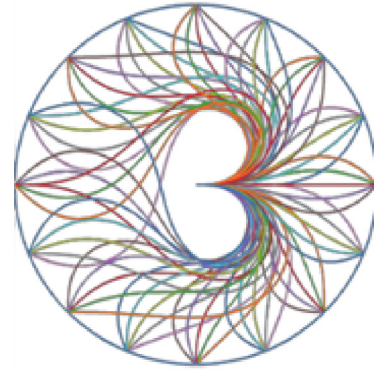
Fig. 2. The 2D motion primitives generated from the initial state (0, 0, 0, 0) .
