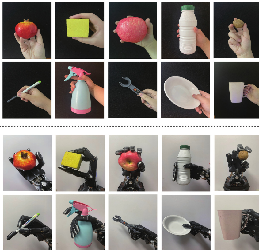
Fig. 1. Demonstration of dexterous manipulation. Human-level dexterous manipulation (top). Human-like dexterous manipulation of anthropomorphic five-fingered hands (bottom).
