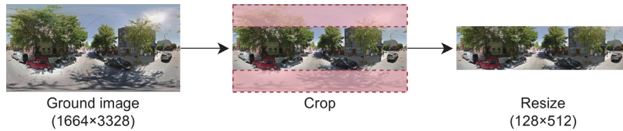
Fig. 6. Process for removing the distorted top and bottom panoramic areas of the ground view image.
