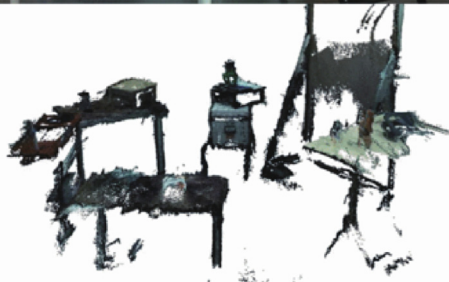
Fig. 2. Dense mapping results on the Valkyrie robot. Reprinted with permission from [15]. Copyright 2017, IEEE.
