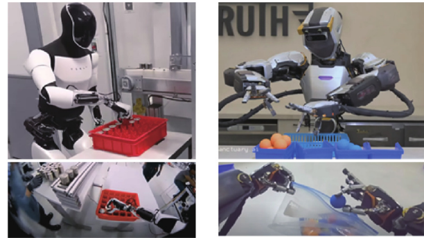
Fig. 10. Visual perception enables advanced semantic understanding. Left: Tesla's Optimus sorting batteries in a factory. Right: Appronik's Apollo inserting colored balls into a sealed plastic bag by opening the seal.
