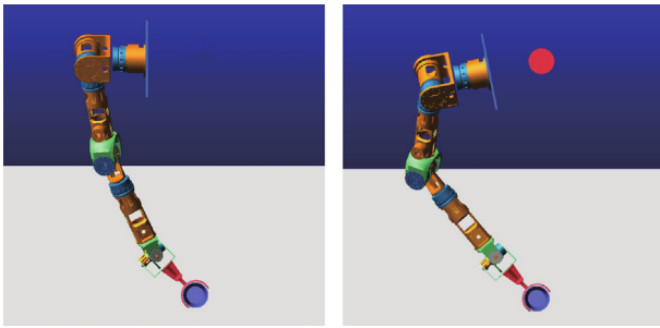
Fig. 7. Configuration comparison of the 7-DOF manipulator without waist joint (left) and the 8-DOF manipulator with waist joint (right).
