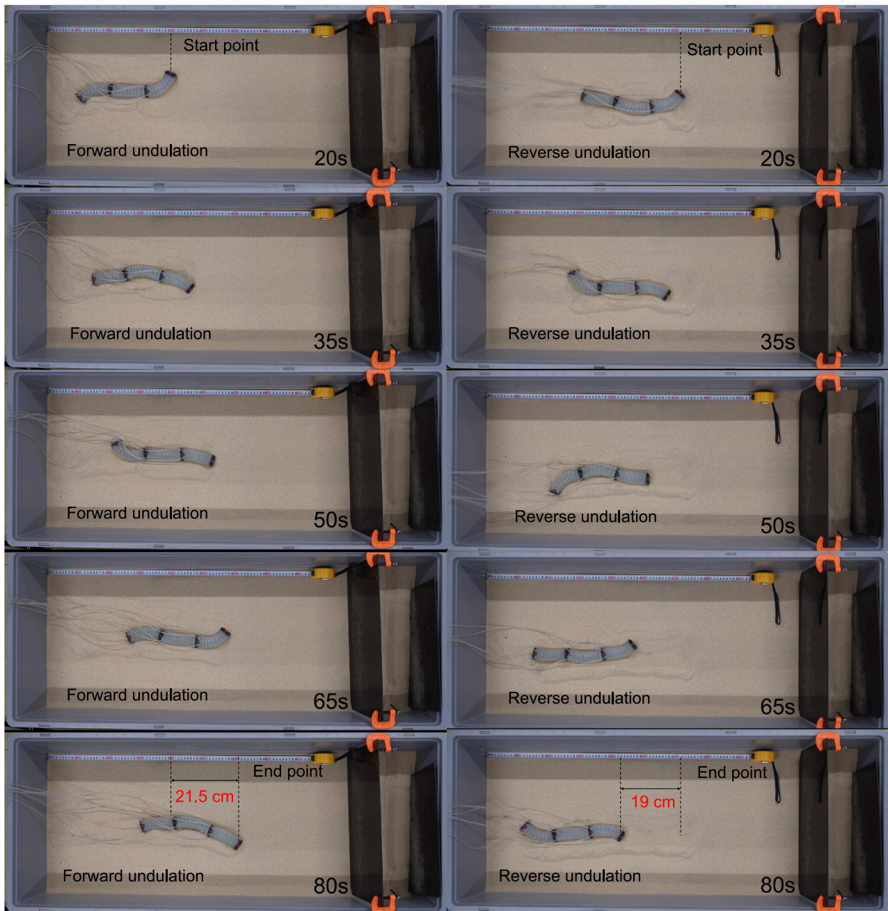
Fig. 11. Illustration of forward and reverse undulation processes driven at 0.55 MPa.
