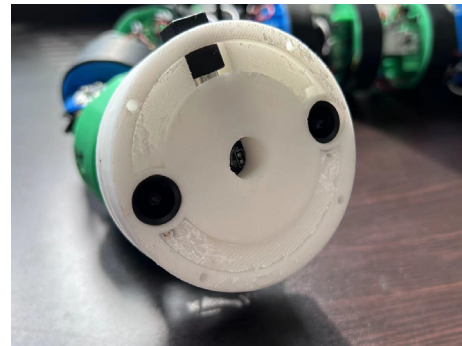
Fig. 3. Snake robot head's 3D-printed housing for mounting binocular camera (without shield).
