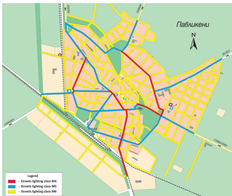
Figure 6. Lighting classification of the street network in the town of Pavlikeni in accordance with EN 13201
