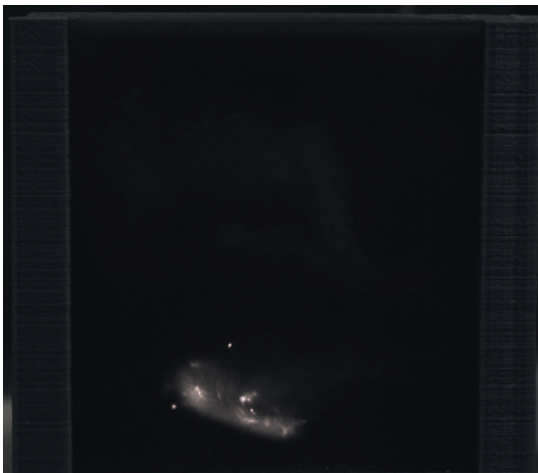
Figure 5. The pyrolysis stage in the deflagration process of cotton floc
