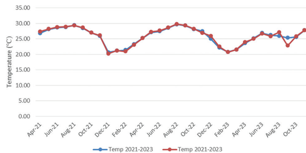
Figure 5. Temperature (Temp) values of treated wastewater from the 10 million liters-per-day sewage treatment plant at Bambianwali (2021 – 2023)
