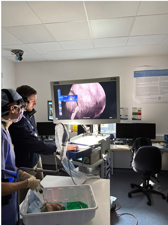
Fig. 1. Karl Storz Rubina® lens system and IMAGE1 S™ technology. During the injection of ICG into the bypass graft, the light emitted by the laser device at 806 nm and 2.0 W excites the fluorophore and the fluorescent emitted light is captured by an infrared-sensitive charge-coupled device (CCD) camera system. The image is clearly displayed in a 4K monitor with the opportunity to obtain information about the intensity of the fluorescent signal (intensity map) and a pure modality of near infrared (monochromatic) to distinguish the contour of the anatomical structure. The possibility to register the fluorescent signal assures the quantification of parameters which are helpful for the stenosis measurement and the control of quality of graft-coronary anastomosis. ICG, indocyanine green. The persons approved the use of this photograph for publication.
