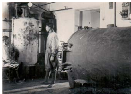
Fig. 2. Autoclave sterilization of culture media and disposal of processed material, the 1940s.
