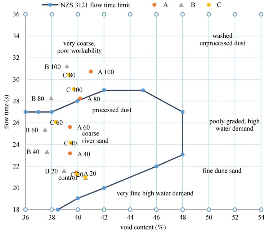
Fig. 5 Flow cone test results.
