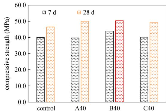
Fig. 13 Compressive strengths of concrete with 40% FCA types A, B, and C.
