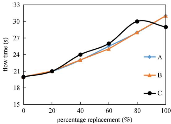
Fig. 6 Variation of flow time with the percentage of FCA.
