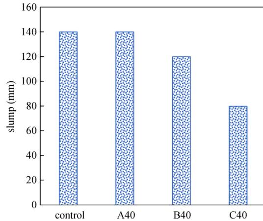
Fig. 10 Variation of slump with the percentage of FCA type C.
