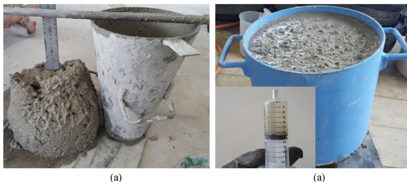
Fig. 4 Tests to determine fresh concrete properties: (a) slump test; (b) bleeding test.
