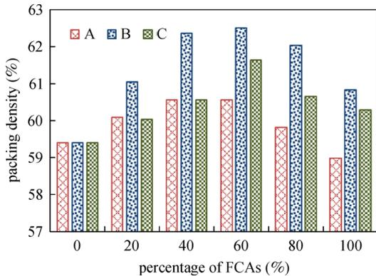
Fig. 8 Variation of packing density with the percentage of FCA.
