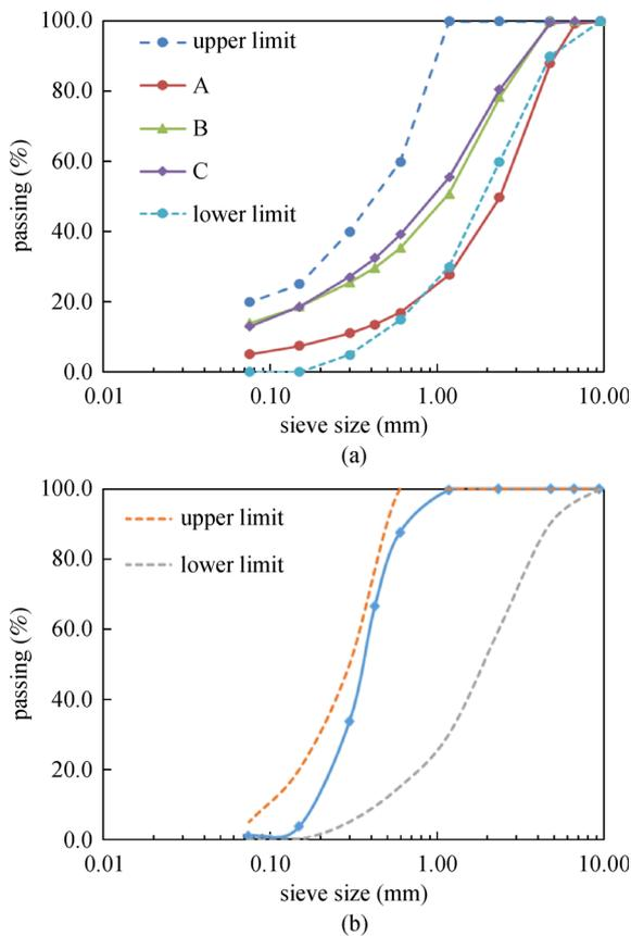
Fig. 3 Particle size distributions of (a) FCAs (A: granophyre, B: basalt, and C: granite); (b) natural sand.
