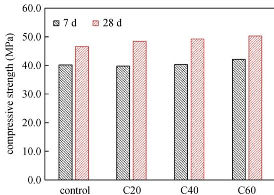
**Fig. 14** Variation of compressive strength with the percentage of FCA type C.
