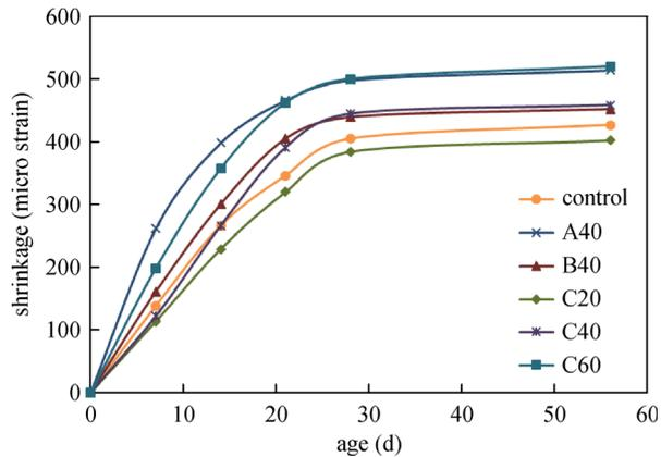
Fig. 16 Variation of drying shrinkage with the age.
