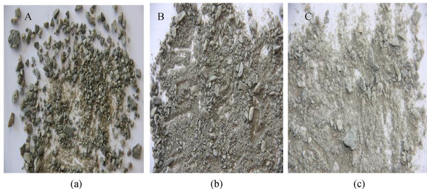
**Fig. 1** Physical appearances of FCAs. (a) Granophyre; (b) basalt; (c) granite.
