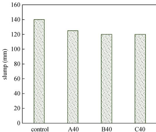
Fig. 9 Slumps of concrete containing 40% FCAs types A, B, and C.
