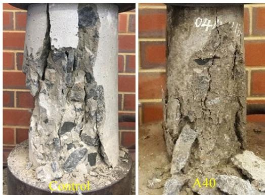
**Fig. 15** Variation of failure pattern between control samples with FCA concrete.
