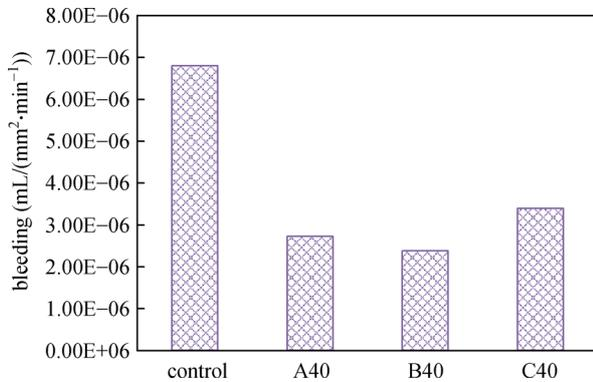
Fig. 11 Bleeding of different concrete mixtures.
