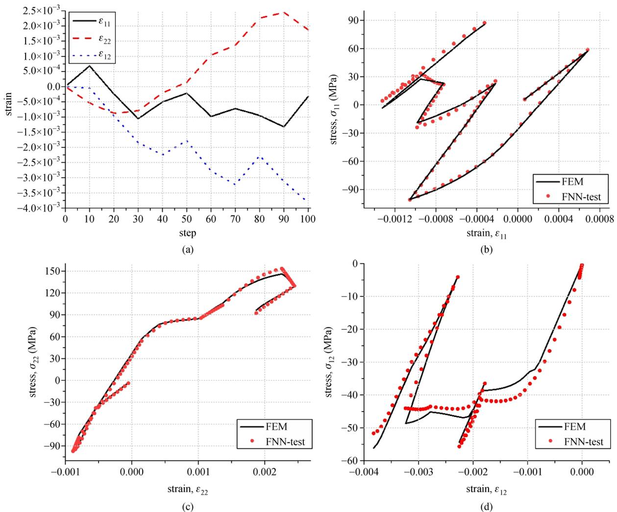
Fig. 13 One loading path and corresponding stress-strain curves in the test set. (a) The loading paths; (b) the stress-strain curves ( $\sigma_{11}$ - $\epsilon_{11}$ ); (c) the stress-strain curves ( $\sigma_{22}$ - $\epsilon_{22}$ ); (d) the stress-strain curves ( $\sigma_{12}$ - $\epsilon_{12}$ ).
