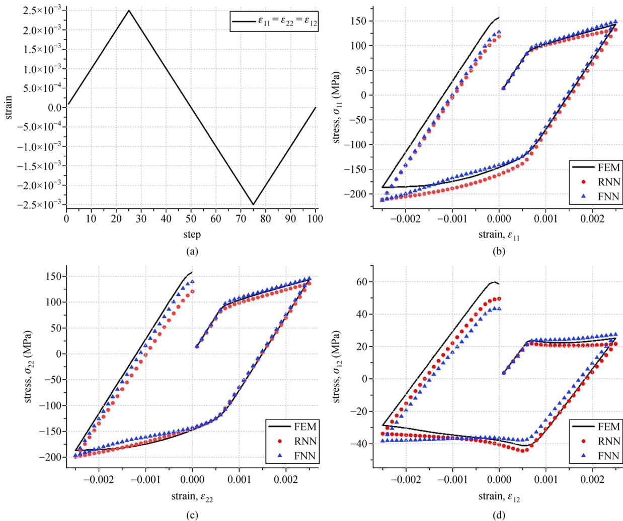
**Fig. 16** First loading path and corresponding stress-strain curves. (a) The loading paths; (b) the stress-strain curves ( $\sigma_{11}$ - $\epsilon_{11}$ ); (c) the stress-strain curves ( $\sigma_{22}$ - $\epsilon_{22}$ ); (d) the stress-strain curves ( $\sigma_{12}$ - $\epsilon_{12}$ ).
