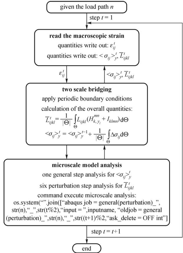
Fig. 2 Flow chart of offline multiscale computation using ABAQUS.
