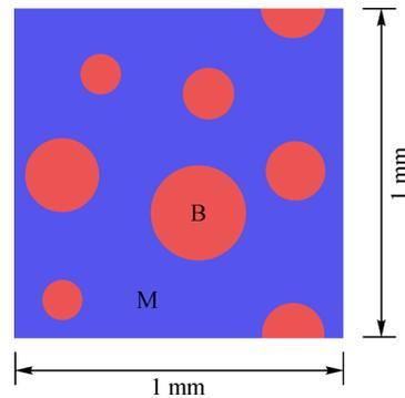
Fig. 9 Two-dimensional RVE model.
