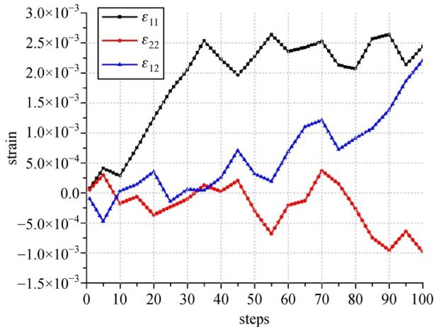
Fig. 11 The macroscopic strain components of different time steps.
