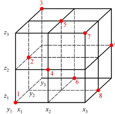
Fig. 8 9 experimental points selected from 27 test points with orthogonal array  $L_9(3^4)$ .
