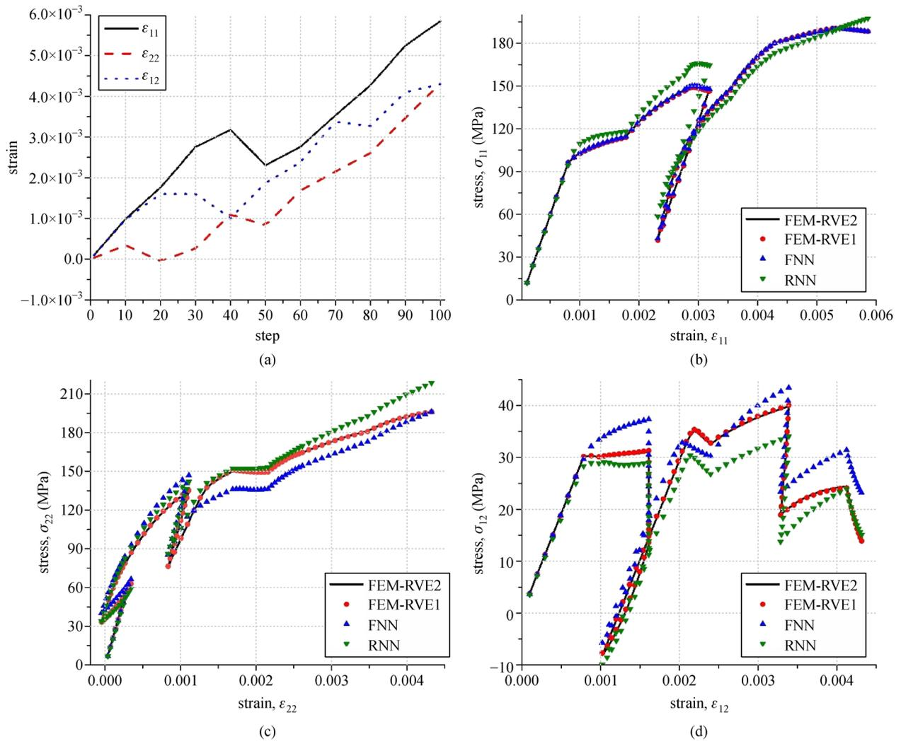
**Fig. 20** A loading path and corresponding stress-strain curves. (a) The loading paths; (b) the stress-strain curves ( $\sigma_{11}$ - $\epsilon_{11}$ ); (c) the stress-strain curves ( $\sigma_{22}$ - $\epsilon_{22}$ ); (d) the stress-strain curves ( $\sigma_{12}$ - $\epsilon_{12}$ ).
