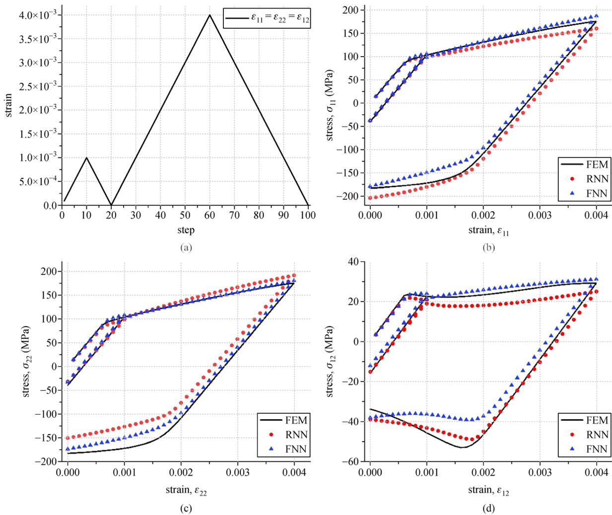
**Fig. 18** Third loading path and corresponding stress-strain curves. (a) The loading paths; (b) the stress-strain curves ( $\sigma_{11}$ - $\epsilon_{11}$ ); (c) the stress-strain curves ( $\sigma_{22}$ - $\epsilon_{22}$ ); (d) the stress-strain curves ( $\sigma_{12}$ - $\epsilon_{12}$ ).
