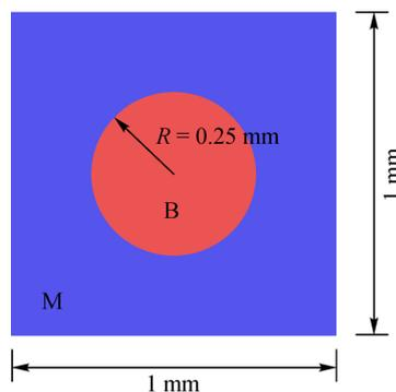
**Fig. 19** Two-dimensional RVE model (RVE2).
