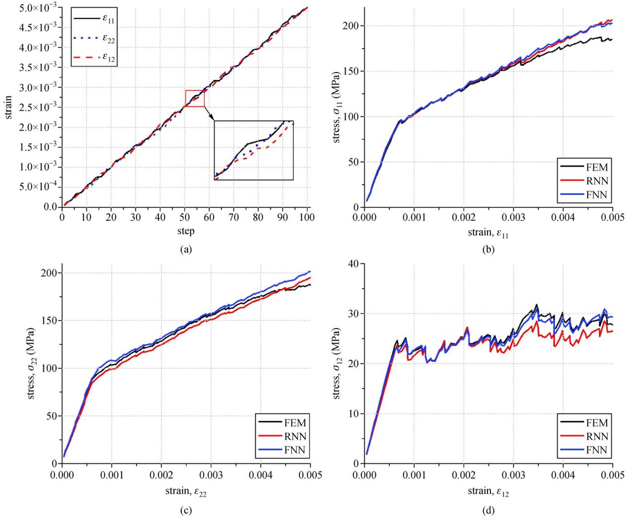
**Fig. 17** Second loading path and corresponding stress-strain curves. (a) The loading paths; (b) the stress-strain curves ( $\sigma_{11}$ - $\varepsilon_{11}$ ); (c) the stress-strain curves ( $\sigma_{22}$ - $\varepsilon_{22}$ ); (d) the stress-strain curves ( $\sigma_{12}$ - $\varepsilon_{12}$ ).
