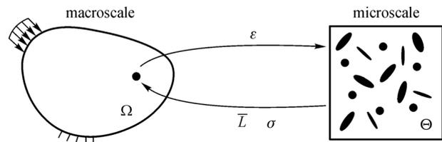
Fig. 1 The computational homogenization scheme.
