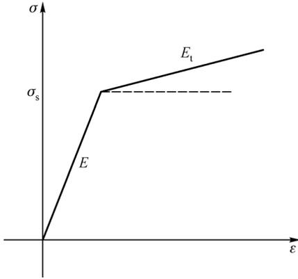
Fig. 10 The isotropic hardening law model.
