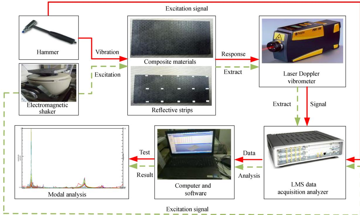
**Fig. 2** Modal test chart of composite material.
