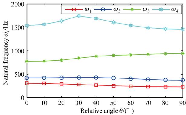
**Fig. 9** Variation of natural frequencies of materials with relative layer angle.
