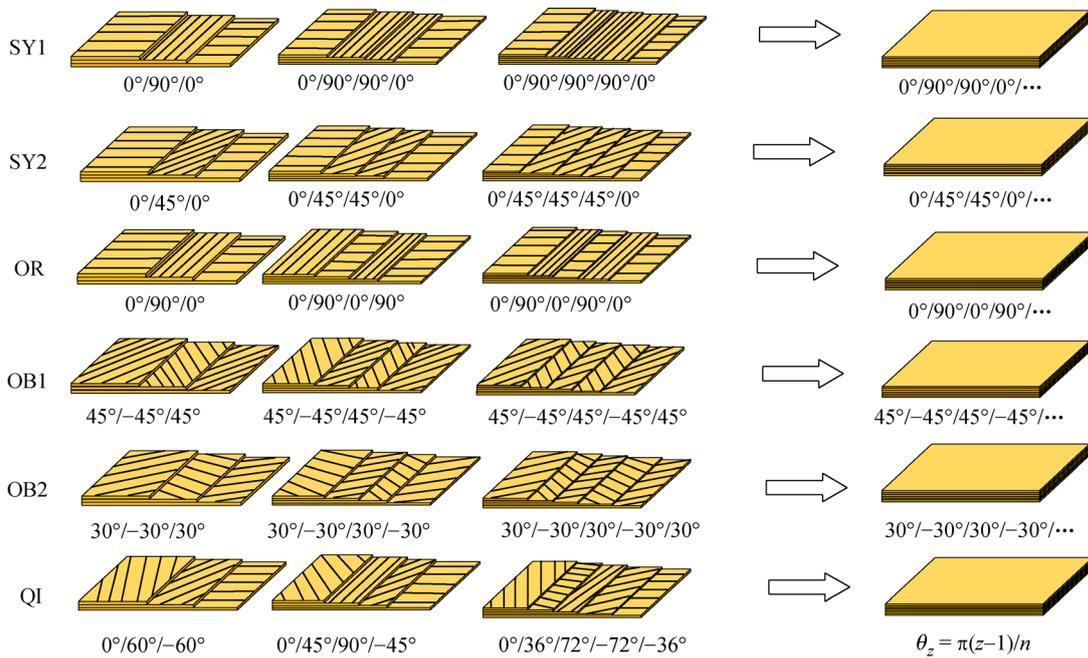
Fig. 10 Laminated composite materials with different structures.
