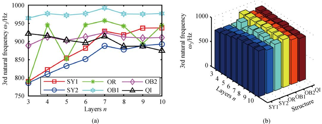
Fig. 13 Effects of different structures on the third-order natural frequency. (a) 2D curve graph; (b) 3D histogram.
