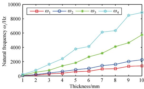
**Fig. 7** Variation of natural frequencies of materials with thickness.
