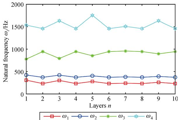
Fig. 5 Effect of the number of layers on the natural frequencies of composites.
