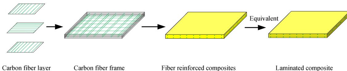
Fig. 1 Production process of fiber-reinforced composites.
