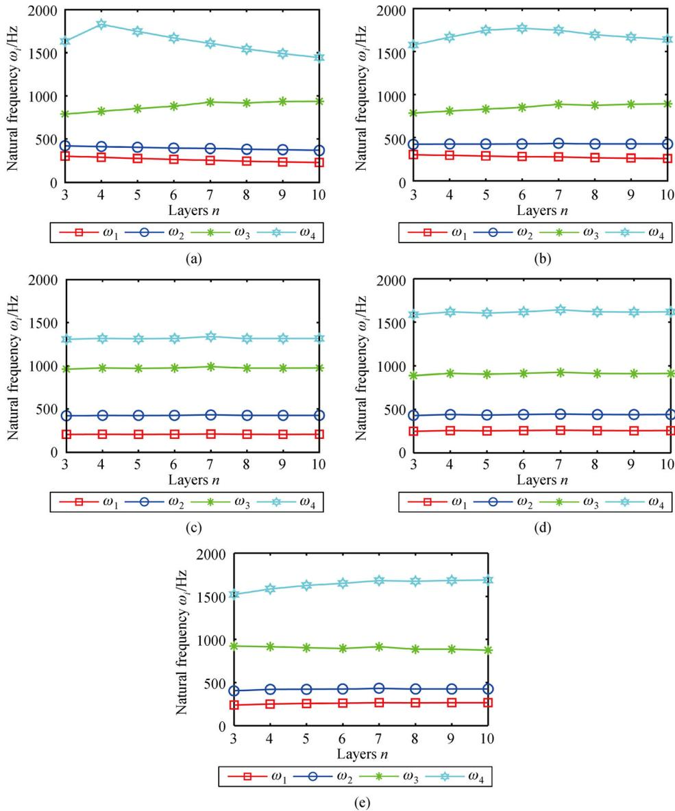
Fig. 15 Effects of the number of layers on the natural frequencies of different structures. (a) SY1; (b) SY2; (c) OB1; (d) OB2; (e) QI.
