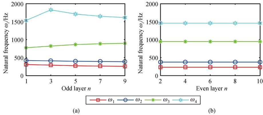
**Fig. 6** Effect of odd and even numbers of layers on the natural frequencies of composite materials. (a) Odd-numbered layers; (b) even-numbered layers.
