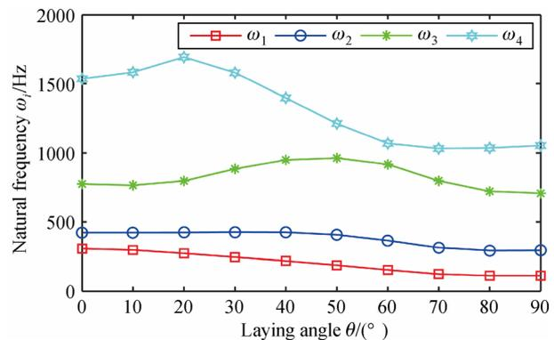
**Fig. 8** Variation of natural frequencies of materials with layer angle.
