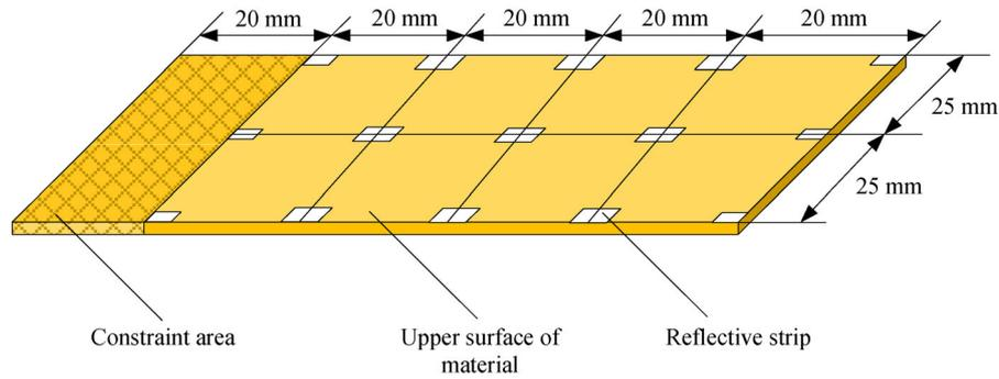
**Fig. 3** Simplified diagram of the distribution of laser reflection strips.
