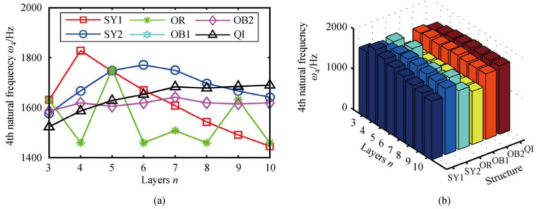
Fig. 14 Effects of different structures on the fourth-order natural frequency. (a) 2D curve graph; (b) 3D histogram.
