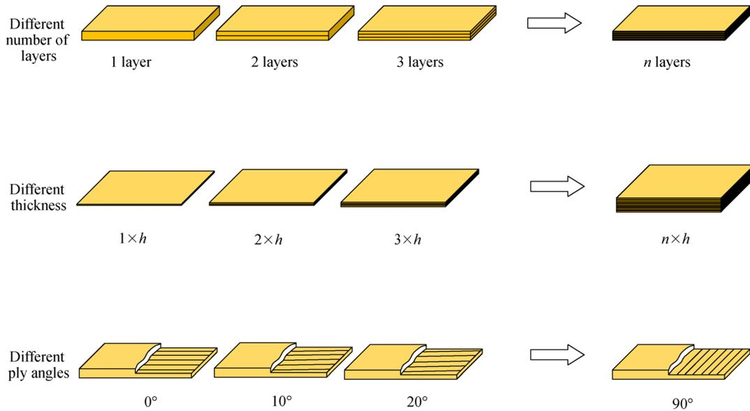
Fig. 4 Laminated composite materials with different structures.
