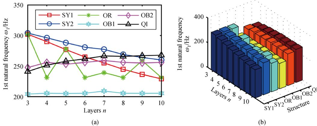
Fig. 11 Effects of different structures on the first-order natural frequency. (a) 2D curve graph; (b) 3D histogram.
