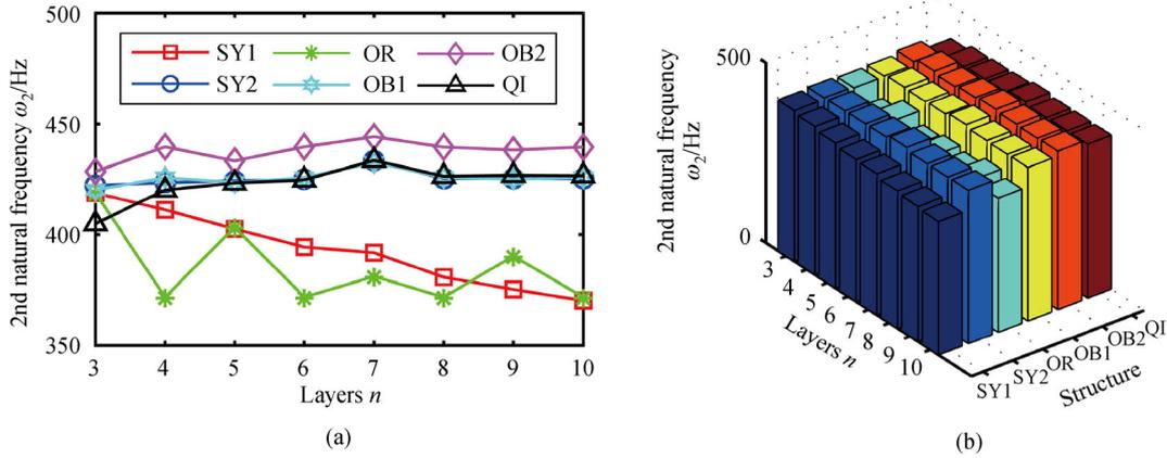
Fig. 12 Effects of different structures on the second-order natural frequency. (a) 2D curve graph; (b) 3D histogram.
