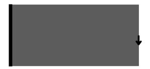
Fig. 1 Design domain and boundary condition of the cantilever problem (size:  $100 \times 50$ )
