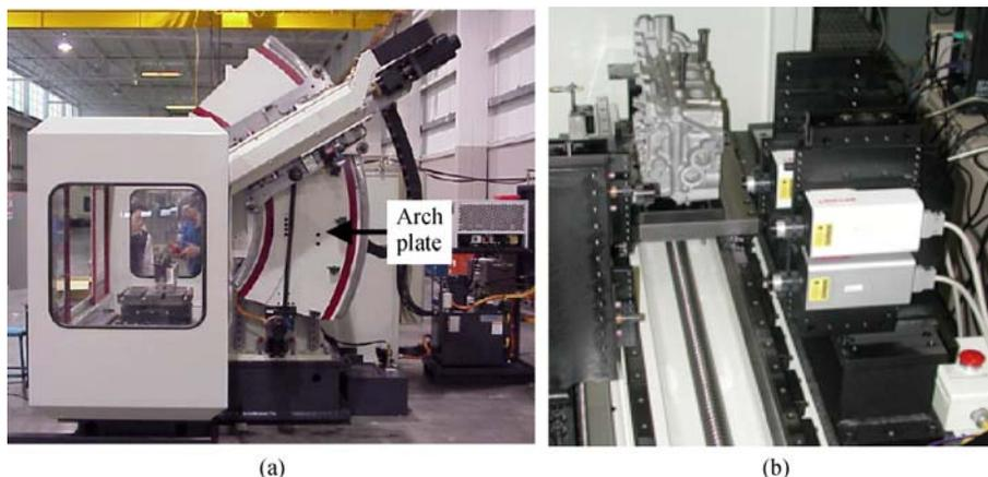
**Fig. 2** Reconfiguration machine tool (RMT) and reconfigurable inspection machine (RIM) developed at the ERC-RMS. (a) RMT; (b) RIM
