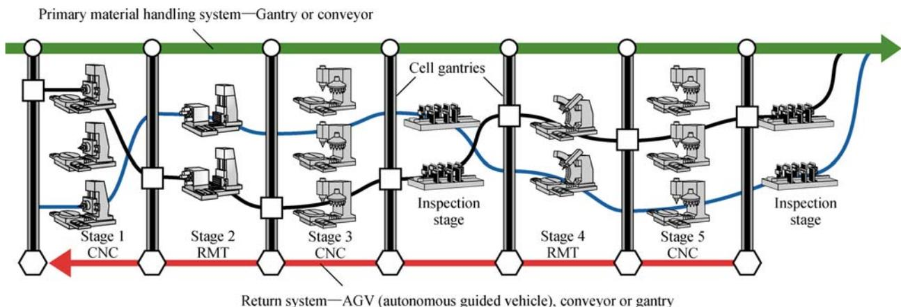
Fig. 5 A futuristic RMS configuration with RIMs and a return conveyor
