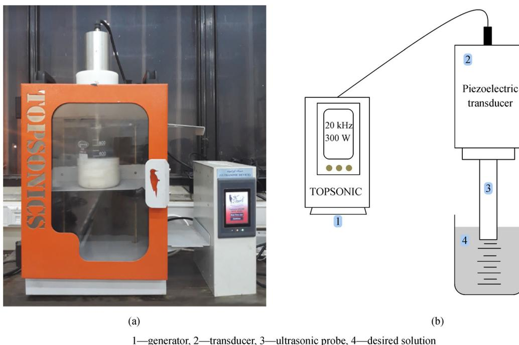
**Fig. 1** Experimental set-up for ultrasound-assisted emulsification process for production of emulsion fuels.
