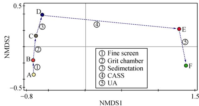
**Fig. 3** Non-metric multidimensional scaling of ARG across the wastewater treatment process (A, B, C, D, E, F represent the sampling locations, ①, ②, ③, ④, and ⑤ represent the treatment processes).
