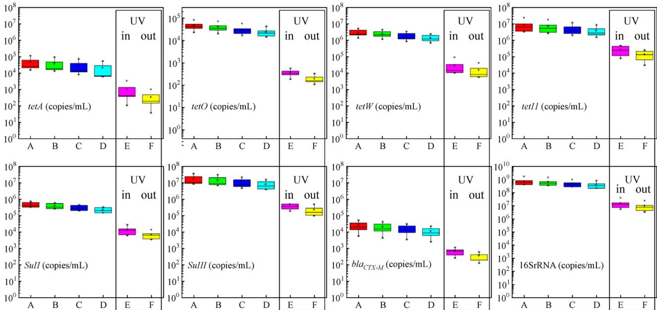
**Fig. 2** Distribution of ARGs in the wastewater under different treatment processes (A, B, C, D, E, F represent the sampling locations after the coarse screen, the fine screen, the grit chamber, the sedimentation tank, CASS, and UV disinfection, respectively).
