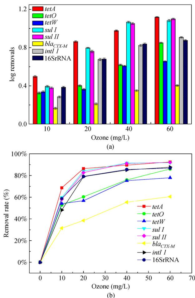
Fig. 4 Removal of ARGs by ozone disinfection.
