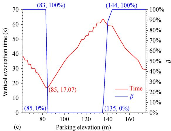
**Fig. 11** Relationship among the parking elevation, evacuation time and ratio  $\beta$  (the number of evacuee is set as (a) 225, (b) 125 and (c) 50).
