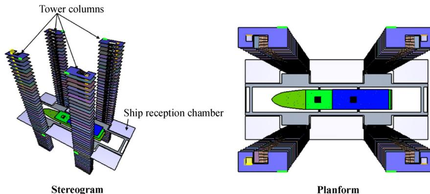
Fig. 1 Structure of the ship lift.
