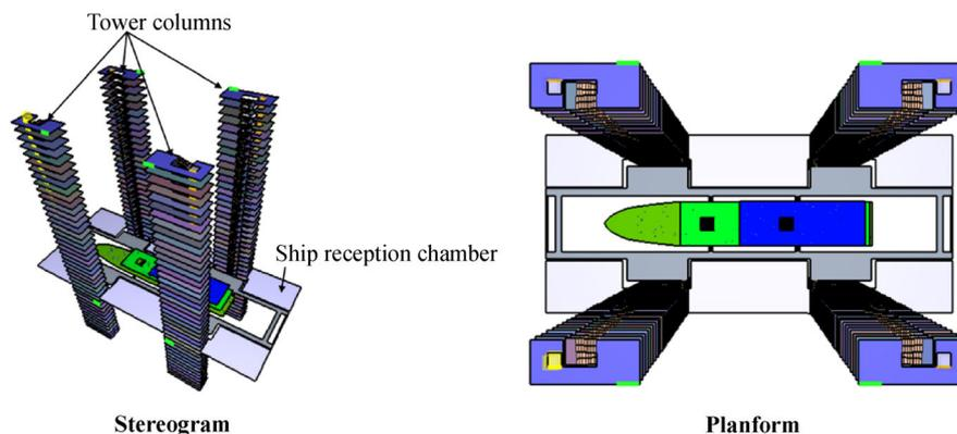
Fig. 1 Structure of the ship lift.
