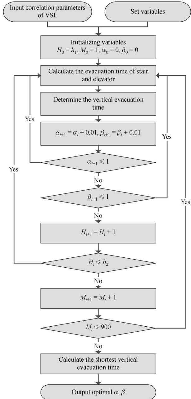
Fig. 5 Simulation process flow.
