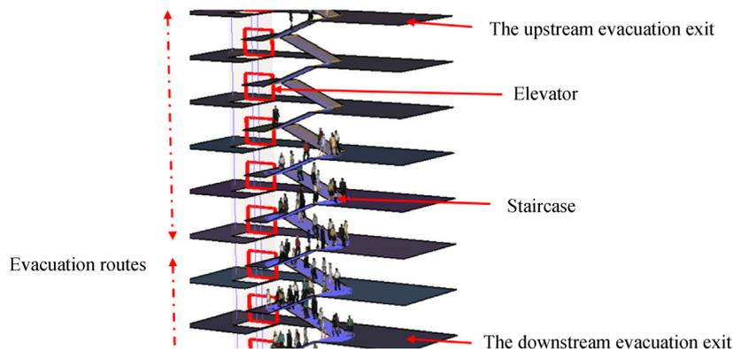
**Fig. 2** Evacuation routes (color blue represents the evacuation trajectory of people on staircases and elevators).
