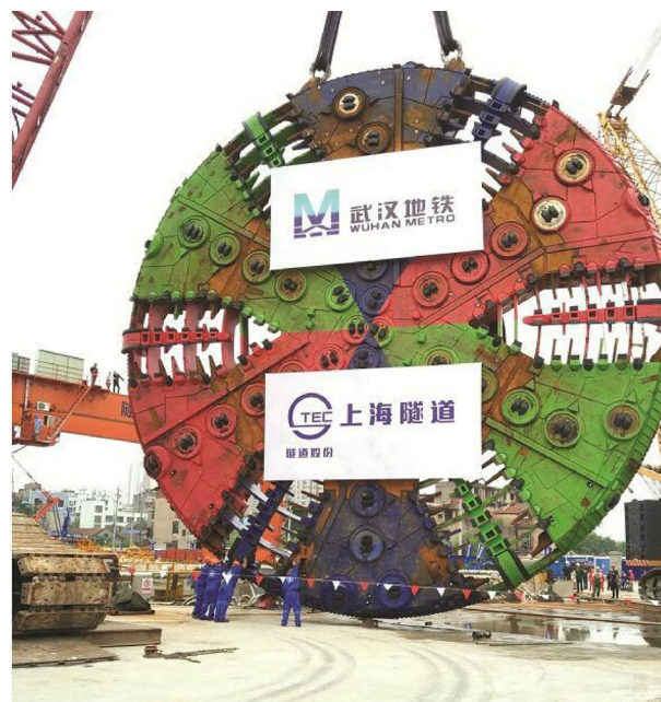
Fig. 2 Super-large-diameter cutter head of shield tunneling machine in Sanyang Road Cross-river Tunnel Project
