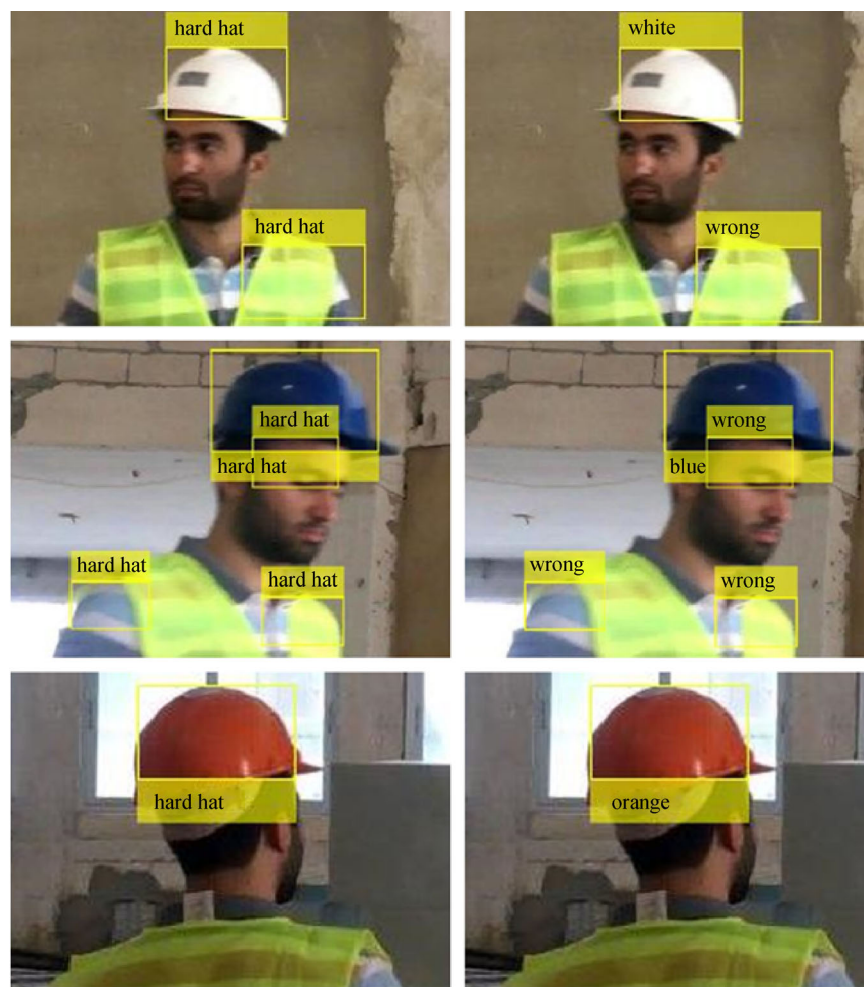
Fig. 14 Hardhat detection results for positive images: (a) cascade object detector and (b) cascade object detector combined with color-based segmentation
