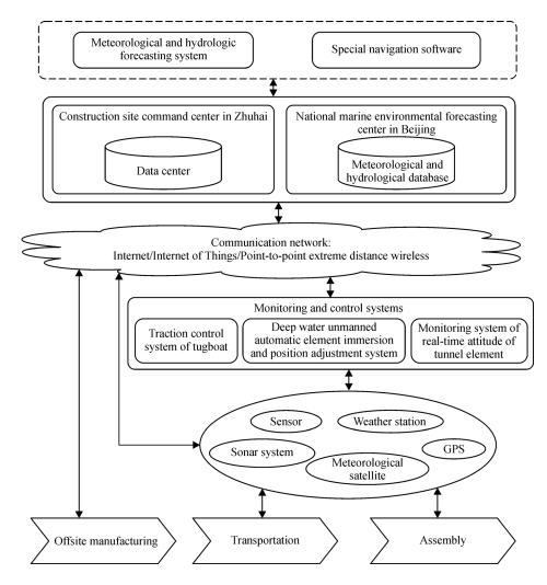
Fig. 3 System framework of smart construction site in HZMB project
