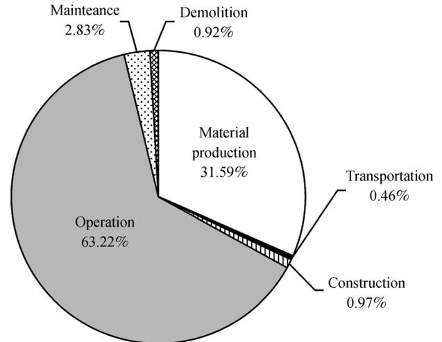
Fig. 3 Carbon emissions from the various building life cycle stages
