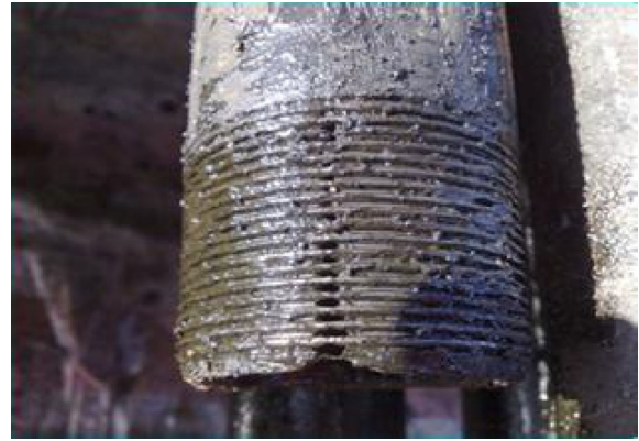
Figure 2. Screw thread damage.
