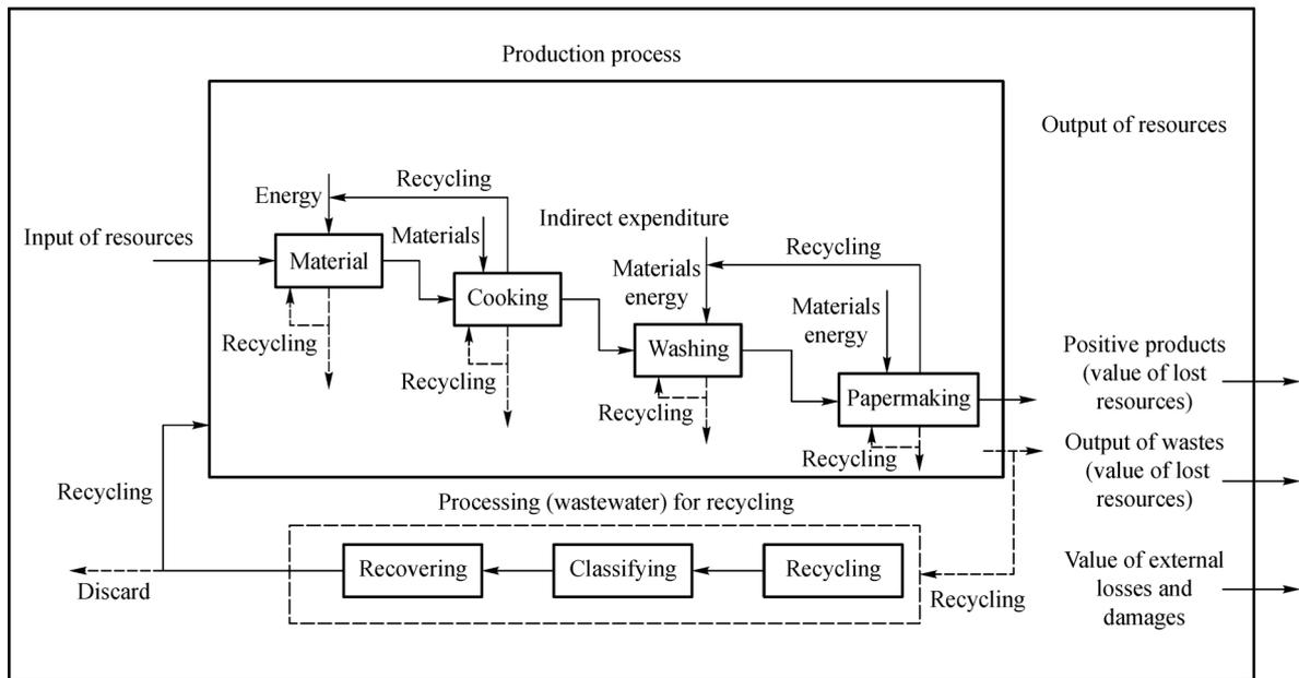
Figure 2. The resource transfer of the papermaking enterprise based on the value flow analysis.
