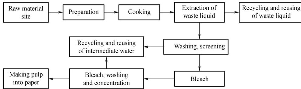
Figure 1. The production process of the papermaking enterprise in which plant fibers are used as raw materials.
