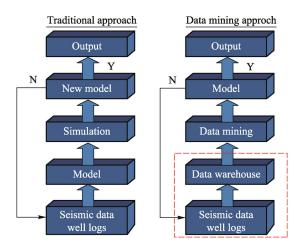
*Figure 4*. Traditional approach vs. data mining approach in petroleum exploration engineering.
