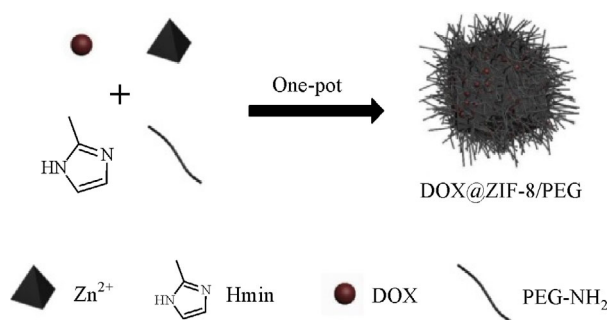
Fig. 8 The preparation of DOX@ZIF-8/PEG via one-pot method. Reprinted with permission from ref. [83]. Copyright 2019, Elsevier.
