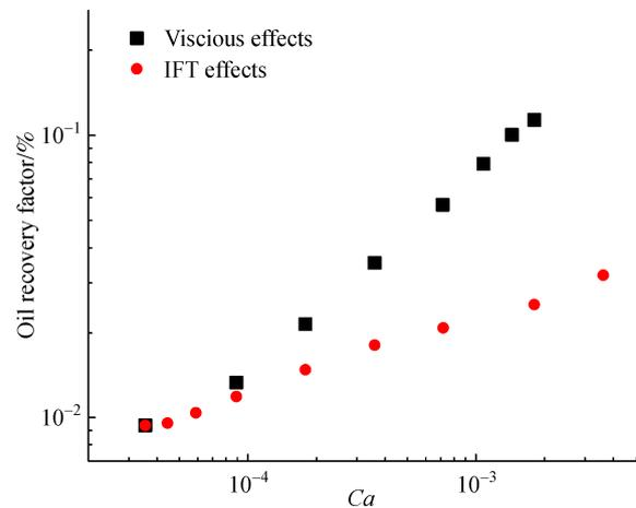
**Fig. 7** Viscosity and IFT effects on oil recovery factor.
