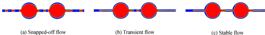
**Fig. 11** An example of the three flow regimes: (a) Snapped-off flow with  $Ca = 1.78 \times 10^{-3}$ , (b) Transient flow with  $Ca = 1.78 \times 10^{-3}$ , (c) stable flow regime with  $Ca = 1.78 \times 10^{-2}$ .
