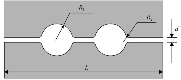
Fig. 1 Schematic view of the two-dimensional pore-throat configuration.
