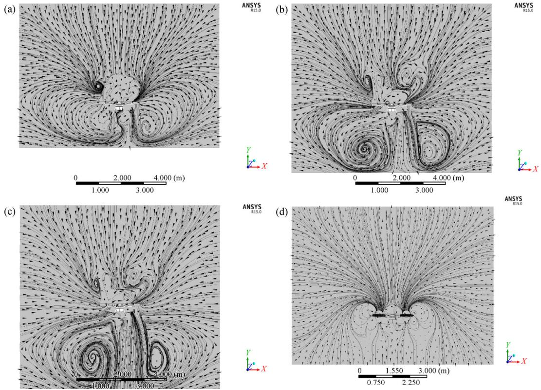
Fig. 9 Streamline vectors for different hovering heights of 2 m (a), 3 m (b), 5 m (c), and the relative boundless height (d)
