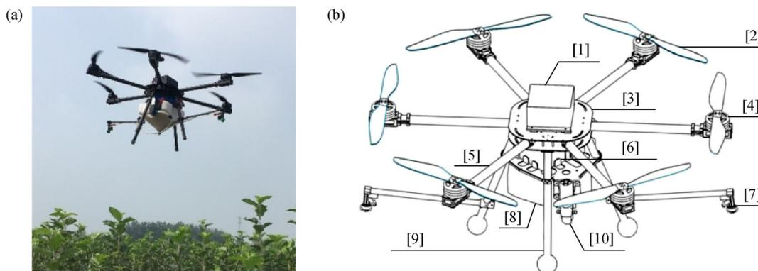
**Fig. 1** JF01-10 plant protection UAV (a) and parts consisting of JF01-10 (b). [1] Flight control box; [2] Propeller; [3] Core circuits; [4] Electric motor; [5] Arm; [6] Battery cabin; [7] Pressure nozzle; [8] Pesticide tank; [9] Landing gear; [10] Pump.
