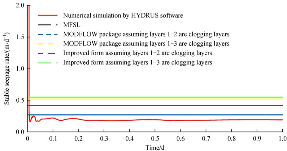
Fig. 4 Comparison of the results of different theoretical methods for calculating stable seepage
