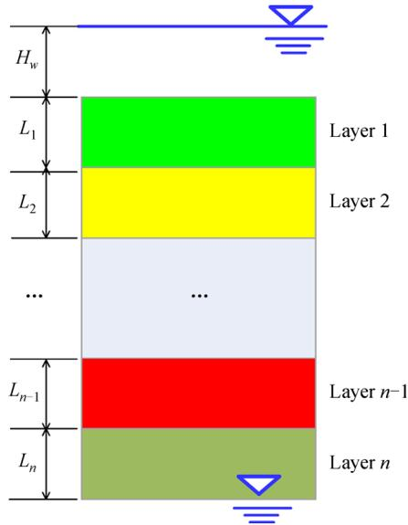
Fig. 2 Schematic of a soil column with  $n$  layers
