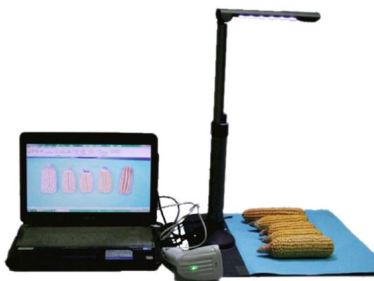
Fig. 2 Corn ear test system developed by China Agricultural University
