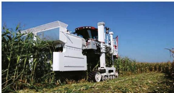
Fig. 4 DuPont Pioneer's large mobile artificial wind tunnel<sup>[22]</sup>
